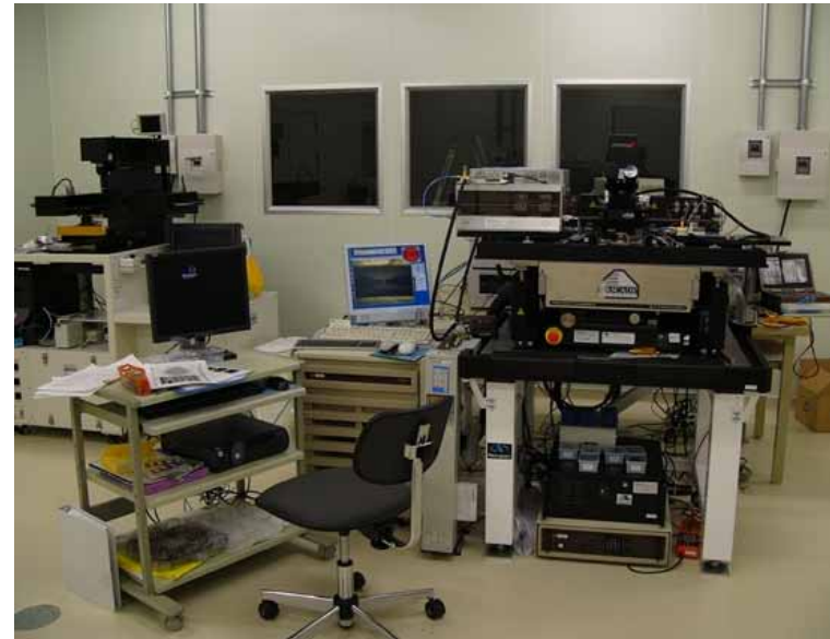
RF measurement system; 8 inch wafer, 40 GHz
